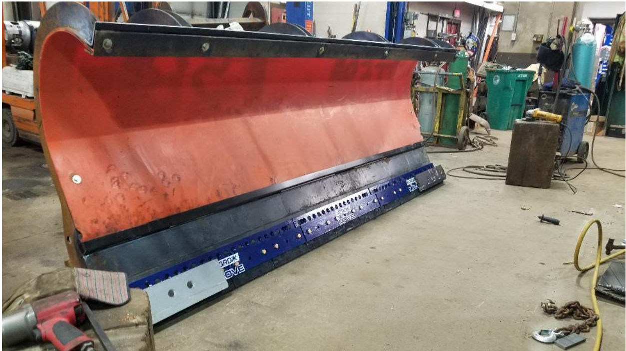
Figure 1 - Rebuilt Plow Frame with Segmental Blade
